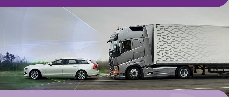
From November 2015 it was mandatory for Forward Collision Warning (FCW) and Automatic Emergency Braking Systems (AEBS) to be fitted to Heavy Goods Vehicles (HGVs) over 7.5 tonnes within the EU. Despite these AEBS, accidents still occur as they may not detect unusual vehicles like highway maintenance vehicles or trailers.
